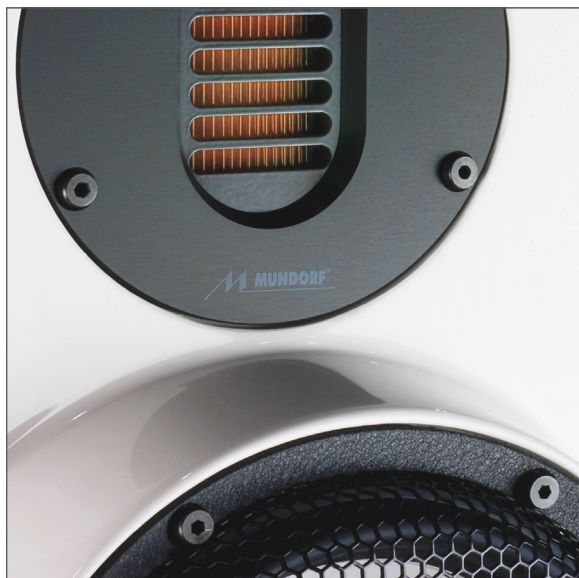
Woofer installed 18 mm forward
